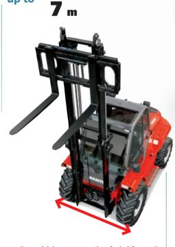
Its **width** ensures the fork-lift truck has better stability for extra safety for lateral loading.
